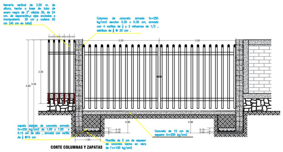
**DETALLE DE ARMADO DE COLUMNAS Y ZAPATAS EN ACCESOS DE CALLE ORQUIDEAS**
